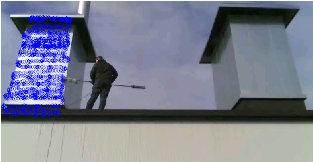
Figure 1: Webcam image of the front part of the left chimney with a selection of measurement points
