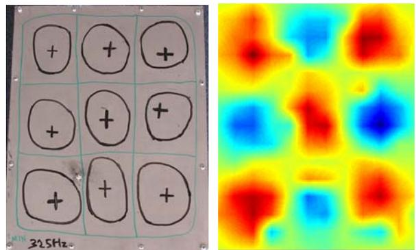
Figure 11: Modes measured at 325Hz with the simple whiteboard marker technique compared with a high resolution (180 points) surface velocity measurement.
