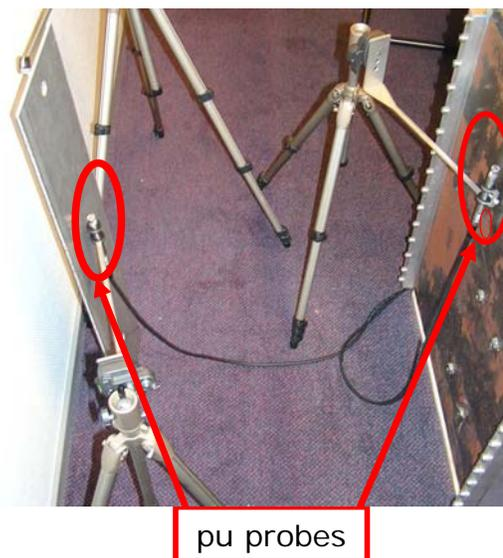
Figure 13: Gong measurement setup.
