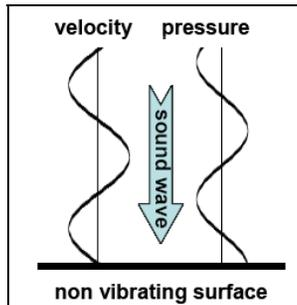
Figure 2: Background noise causes a high sound pressure and a low particle velocity level at a rigid surface.
