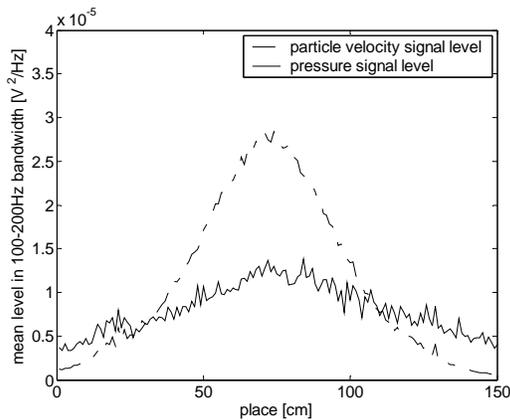
Figure 6: Surface scan without background noise.
