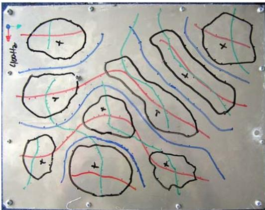
Figure 9: A simple way to find a modeshape at 400Hz. In red and green are the lines of zero lateral velocity shown. In black iso-velocity lines and in blue the lines of zero normal velocity. The black crosses are the points of maximal normal velocity.
