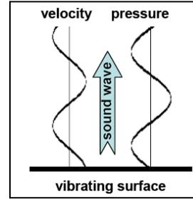
Figure 3: Close by a vibrating structure a high particle velocity level and a low sound pressure level is observed.
