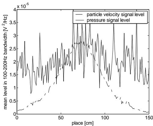
Figure 7: Surface scan with background noise.
