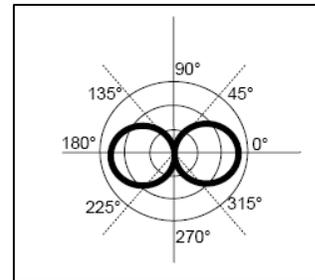
Figure 4: A particle velocity sensor is directional.
