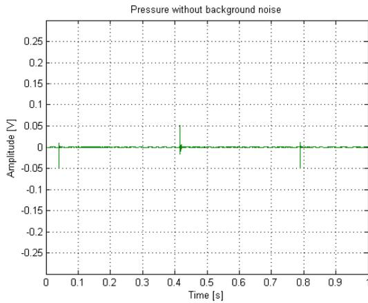
Figure 14: Sound pressure measured close by the miniature loudspeaker (no background noise).
