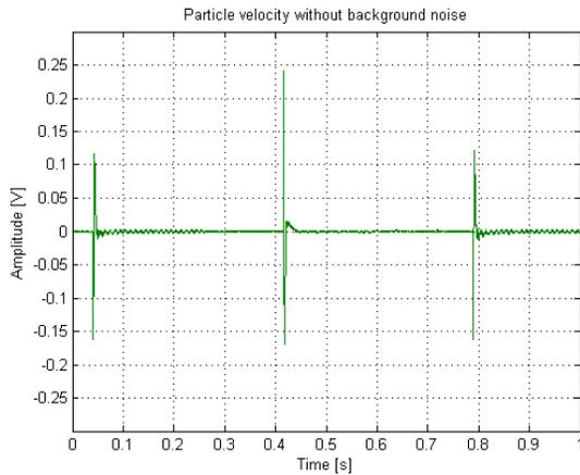
Figure 15: Particle velocity measured close by the miniature loudspeaker (no background noise).
