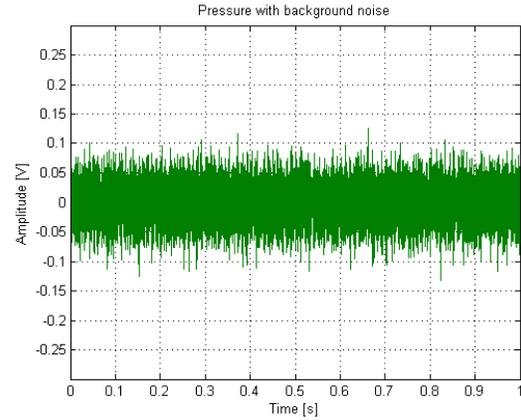
Figure 16: Sound pressure measured close by the miniature loudspeaker (with background noise).
