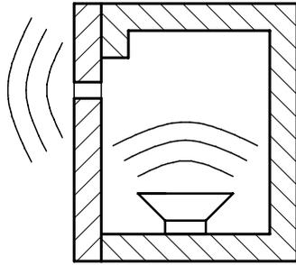
Figure 5: Sound emission from a small hole.
