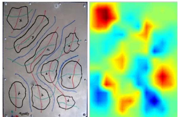
Figure 12: Modes measured at 400Hz with the simple whiteboard marker technique compared with a high resolution (180 points) surface velocity measurement.
