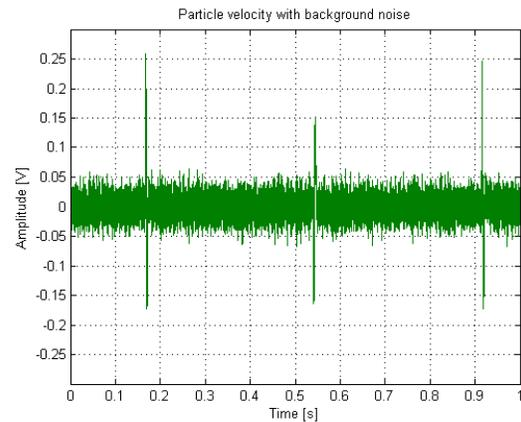
Figure 17: Particle velocity measured close by the miniature loudspeaker (with background noise).
