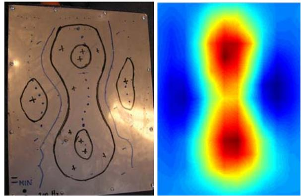
Figure 10: Modes measured at 200Hz with the simple whiteboard marker technique compared with a high resolution (180 points) surface velocity measurement.
