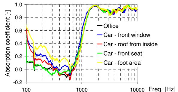
Figure 2. Absorption measurements in a car
