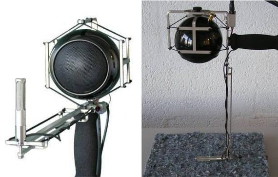
Figure 1. Handheld PU free field impedance setup
