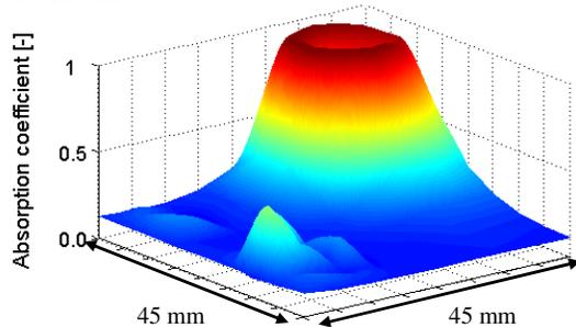
Figure 3. Absorption quarter lambda resonator at 1330Hz
