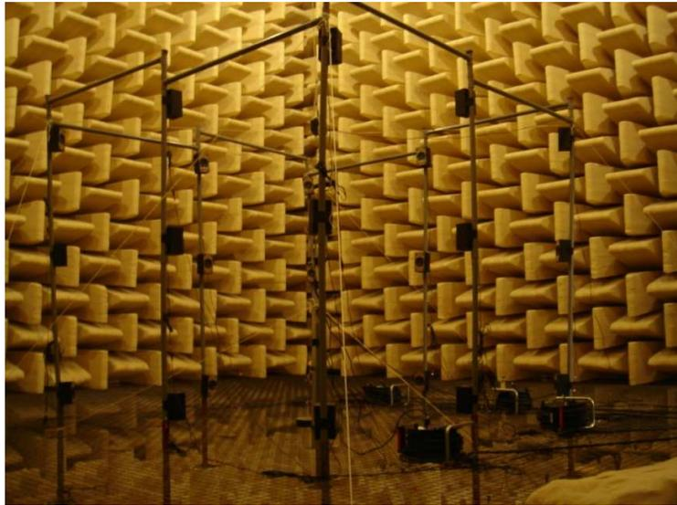
**Figure 2: Setup.** *Twenty-four sources are arranged in a cubic grid of 3x3x3 loudspeakers, where the centre column of loudspeakers is left out.*
