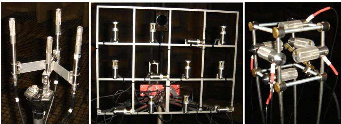
**Figure 3a: Three P-U arrays.** *Left: AVS quad. Middle: Acoustic Camera. Right: velocity gradient array.*
