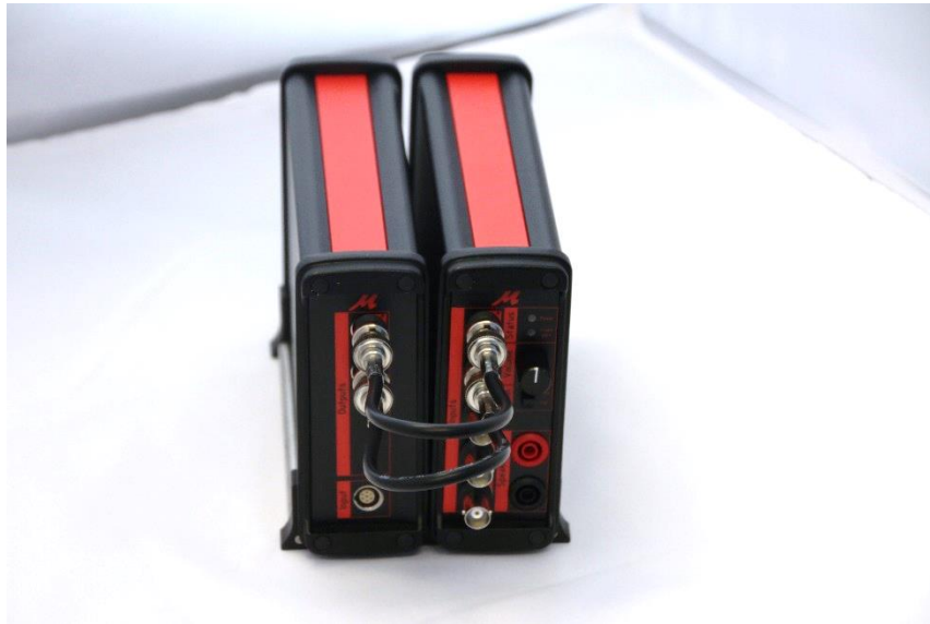
Figure 2. Connect MFPA to Fronted with as many BNC cables as MFPA outputs
