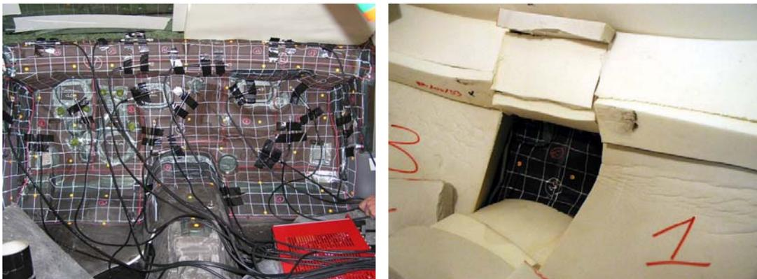
**Fig. 1: Measurement of the engine noise contribution. Left: measurement grid and placement of sound probes. Right: detail of mock up insulation package**
