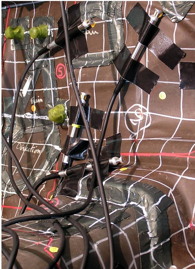
The use of particle velocity based fully integrated p-u sound probes allows the development of new sound power based measurement methods to optimize the acoustical packages for car interiors.
